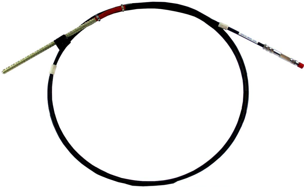
Fig. 2 Extensometer in packed condition, ready for installation, rolled up in a coil of approximately 1.2 m diameter
