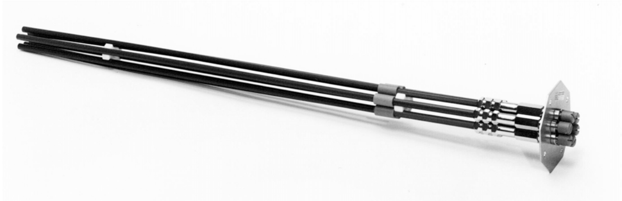
Fig. 3 6-point extensometer with base plate and plastic bracket. Transducers are screwed directly on the measuring head for remote reading.
