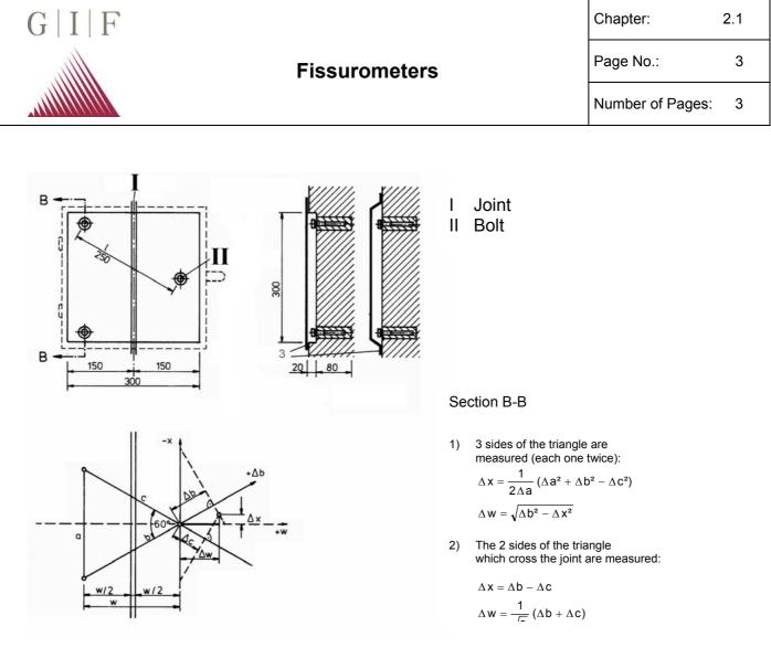
Fig. 2 Displacement measurements with three measurement rods a) Installation drawing; b) Calculation of relative displacement
