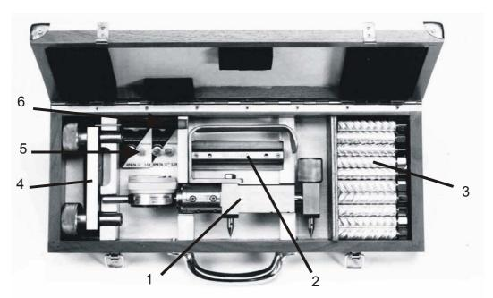
Fig. 1 Mechanical fissurometer type FM 100 with accessories. 1 Fissurometer, 2 Measuring rod type FB 70, 3 Calibration device made of INVAR steel, 4 Setting gauge, 5 Spare batteries for electric dial gauge, 6 Screwdriver for changing the battery
