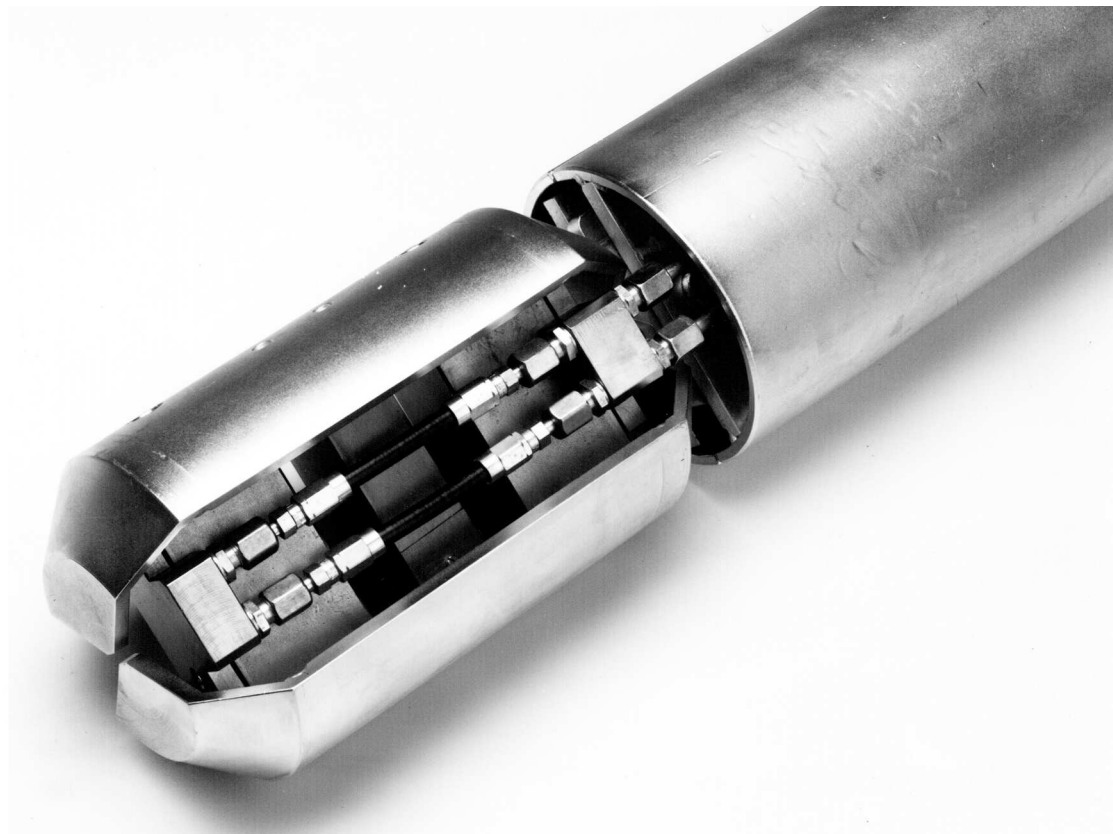
Fig. 1 Ettliger borehole jack ESDS I/146: Loading shells, cylinders and displacement transducers
