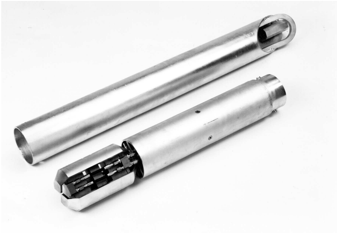
Fig. 2 Ettliger borehole jack ESDS I/146 with sump tube
