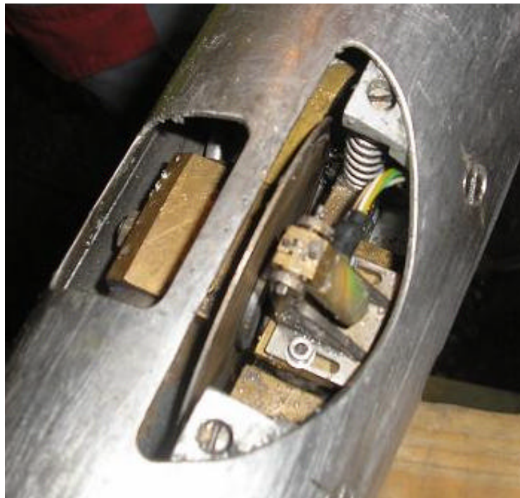
Fig. 2 Strain sensor besides the diamond saw blade
